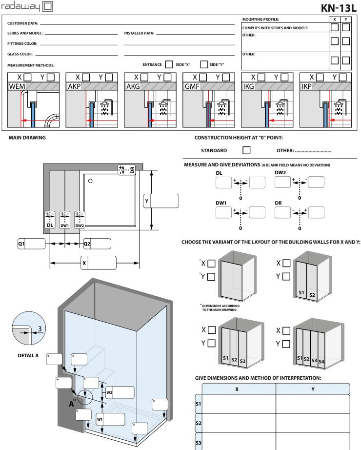
\*INDICATE "0" POINT(S) AND SEPCIFY DEVIATION(S) AS A NEGATIVE VALUE POINT(S) "0" IS/ARE THE HIGHEST POINT(S) ON THE FLOOR / SHOWER TRAY / L-SHAPE WALL CHECK THE FLATNESS AND DESCRIBE ANY CURVES. STANDARD GAP IS 3 MM, CONSIDER INCREASING IT.
