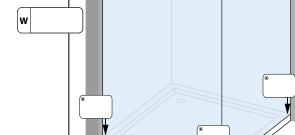
\*INDICATE "0" POINT(S) AND SEPCIFY DEVIATION(S) AS A NEGATIVE VALUE POINT(S) "0" IS/ARE THE HIGHEST POINT(S) ON THE FLOOR / SHOWER TRAY / L-SHAPE WALL
